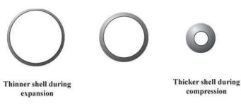
Figure 4: A depiction of the change in mass transfer boundary layer (shell) thickness of a bubble during the expansion and compression cycles of an acoustic wave. The concentration gradient is thus enhanced during bubble expansion.
